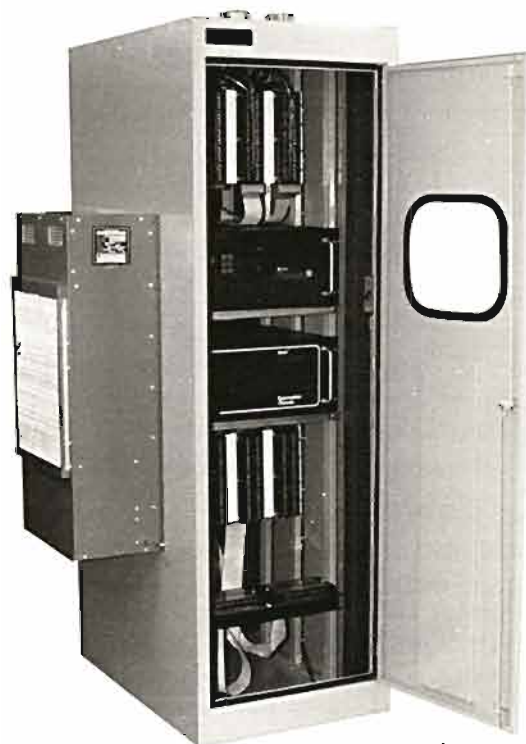
The NEM01 is a special NEMA 12 enclosure for MACSYM products. It provides internal power distribution, cable management, and protection against dust, dirt, and splashing. Its closed-loop air conditioner maintains specified temperature at ambients up to 52°C.
